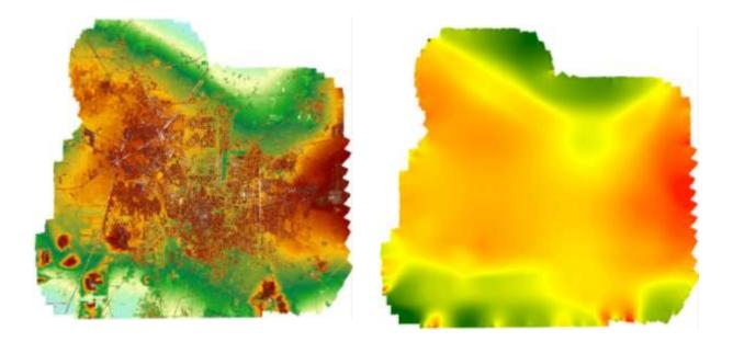
Figure 4 (a & b): Digital Surface Model (5 cm) and Digital Terrain Model (5 cm)
