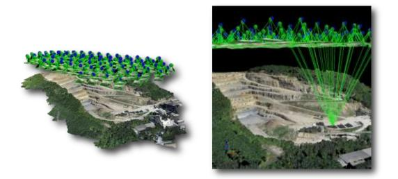
Figure 5. 3D Point Cloud
